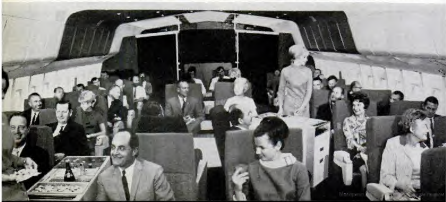
TRISTAR FIRST-CLASS INTERIOR has seats arranged in pairs, eight-foot ceilings, large windows, two aisles
